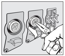
Use pointed nose pliers to withdraw the plastic filter by the bar (see illustration). Clean, put back and secure.
