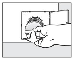
■ Remove the drain filter completely.
